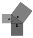
When a triangle has a right angle (90°) and squares are made on each of the three sides, then the biggest square has the **exact same area** as the other two squares put together!
