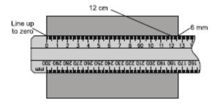
Line the point '0' of the ruler up against what you want to measure or the point where you need to draw a line. In the example we used the end of the piece of paper.
