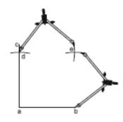
Put the compass point on point 'b' and draw an arc, then set the compass point on point 'd' and draw an arc to cross at 'e'.
